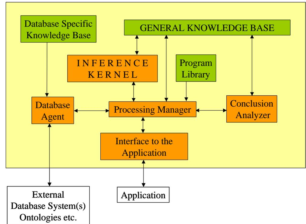
Figure 1: Components of ARIX\_mv. Arrows indicate the data flow between the units.
